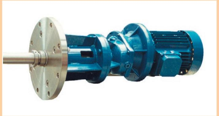
Mixer for side assembling for middle / big sized tanks (100 m<sup>3</sup>) with internal or external mechanical seals, coupling flanges according to UNI – ANSI regulations.
