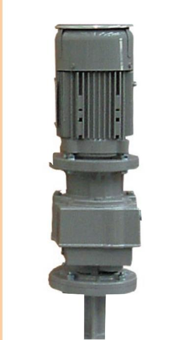
Slow speed mixers with coaxial gearboxes. The speed reducer is of the screw rack type with cylindrical gears, and is coupled to the shaft via a rigid coupling.
