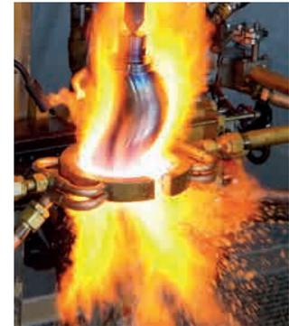
Rotor at flame-hardening process
