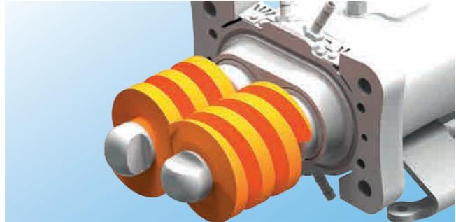
Non-contact feed screw operation, efficient, compact. Developed to reliably convey low to highly viscous, volatile or gaseous products. Its design avoids dead space and stagnation zones. Due to their high speed range, they can be used as a process pump and as a cleaning pump.
