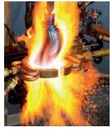
Rotor at flame-hardening process
