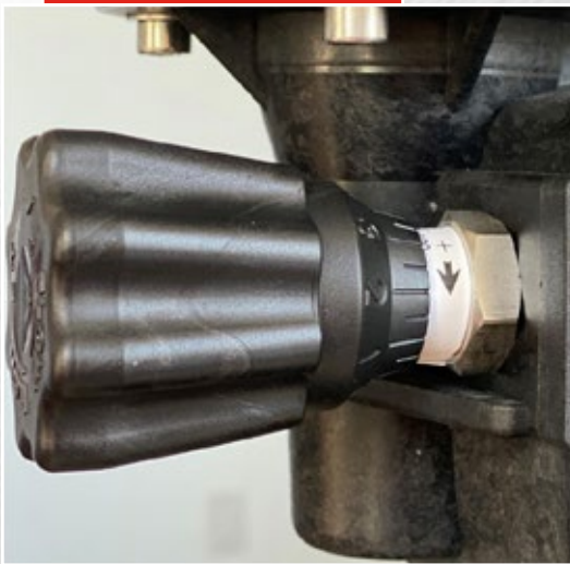
Micrometer stroke adjustment
