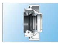
Mechanical seal with bellows
