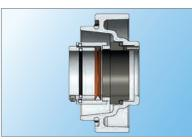
Encapsulated mechanical seal
