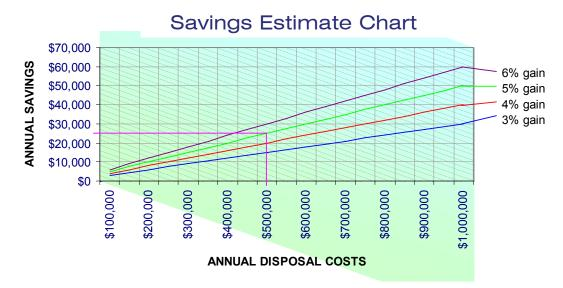
The chart shown above illustrates the savings that are possible using the SIMFLOC 5.0 optimizing system to reduce waste disposal & hauling costs. Find your typical annual costs for hauling and disposal of waste sludge along the bottom of the chart. The four lines represent different gains in sludge solids possible with the SIMFLOC 5.0. The calculated annual savings are shown on the left. The example given is for a 5% gain in efficiency on annual disposal costs of \$500,000. This customer
