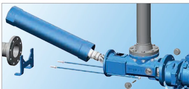
Step 3: Pull the stator and rotor along with the cardan shaft forwards, tip upwards and pull out of the pump housing.
