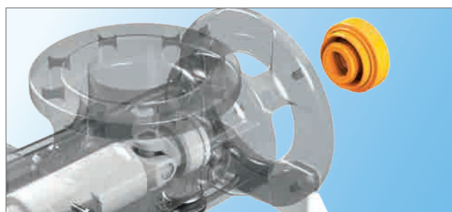
Remove the old seal unit
