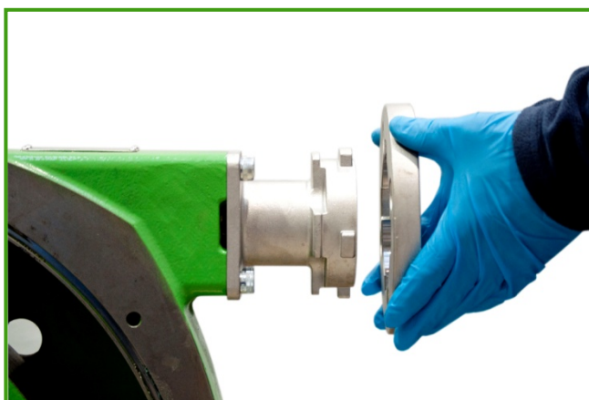
Figure 8 Fitting the port flange
