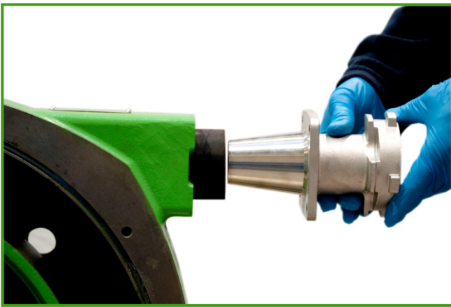
Figure 7 Fitting the port flange-insert
