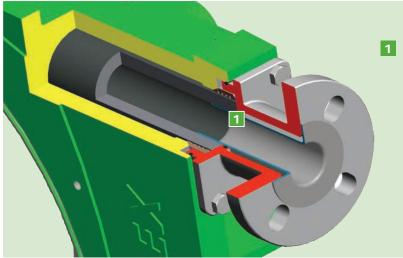
1 When fitted with hygienic flanges (e.g. DIN 11851, Triclamp or RJT) the pump meets EHEDG Standards
