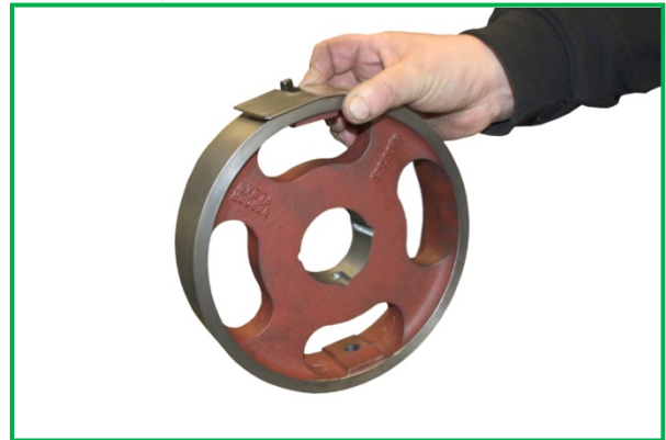
Figure 9 Mounting rotor shims on the rotor (Step 1)
