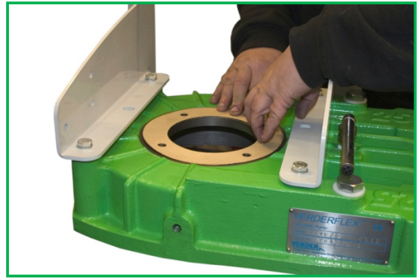
Figure 7 Fitting the drive gasket
