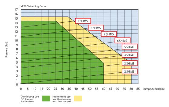
For product temperatures above  $65^{\circ}$ C and/or viscocity's above 2000 mPas use one shim less than shown
