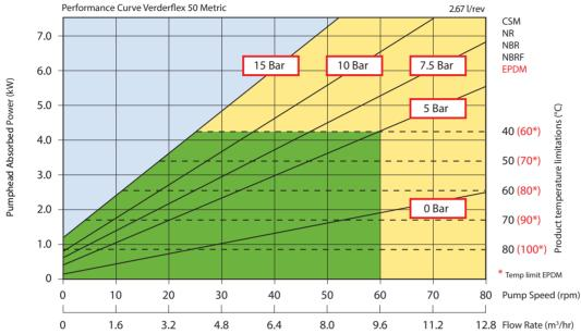
Displacement 2.67 l/revolution, Capacity is speed x 0.16 in m³/hr. Minimum starting torque required: 620 Nm Maximum Peak Power +4%
