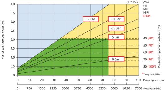
Displacement 1.25 l/revolution, Capacity is speed x 75 in l/hr. Minimum starting torque required: 320 Nm Maximum Peak Power +12%
