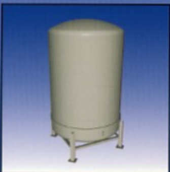
Dished top, and bottom, with elevated steel mounting support. An RTP tank designed for installation above ground supported around the entire circumference with 3 or more legs for tie down.
